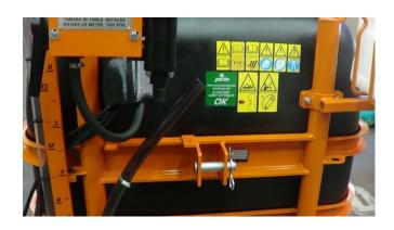
For the J600CHT, locate the two metal tabs next to the top link pin as shown in the picture.
