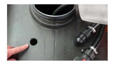
Install the supplied bypass fitting into the new hole in the tank as shown.
