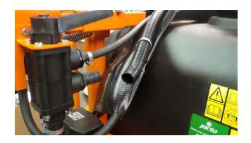
Reinstall the bypass hose to the right side fitting on the electric valve.
