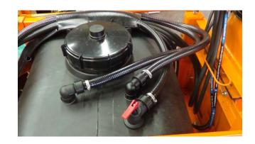
Install the other end of the hose to the bypass fitting on the manual control valve as shown and tighten with a hose clamp
