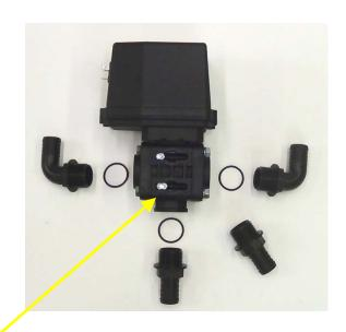
Insert the supplied 5/16" bolts, into the slotted holes on the backside of the electric valve and install the electric valve onto the fabricated metal bracket as shown.
